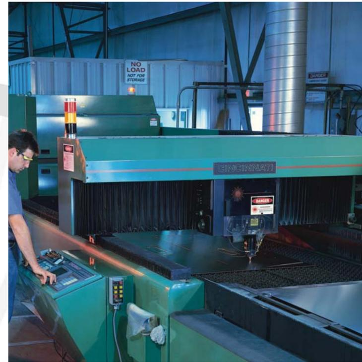
Pictured above: one of two Cincinnati helium-neon laser cutting machines that produce parts to exacting tolerances; below: the 2005 Eureka Brougham Cadillac funeral coach with optional "limousine style" windows.
